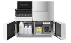
Easy access to place washer, diluent, waste liquid, and waste box in the drawer under the table
